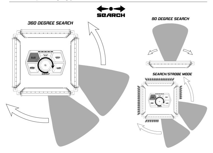
Search Mode allows the user to direct the light where necessary. To activate Search, simply click the Search button. The forward-facing light bars will illuminate and can be controlled via the center turn dial. Turn the dial clockwise to direct right, and counterclockwise to direct left.
